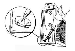
Measuring Voltage at Ionizing Collecting Cell
