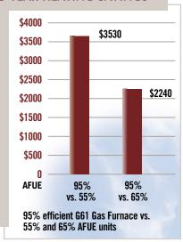
This chart depicts potential energy savings you can expect from the G61 furnace, versus older furnaces with lower efficiency ratings. Criteria used in this example are 2,000 full-load heating hours, with a 60,000 Btuh heating design load and \$1.281 ccf for gas. Your actual savings may vary, depending on the weather patterns in your local area, local fuel rates and your individual lifectule.
