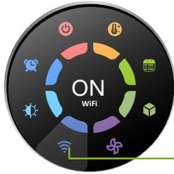
Setting wifi to ON means the thermostat is in wifi pairing state.
