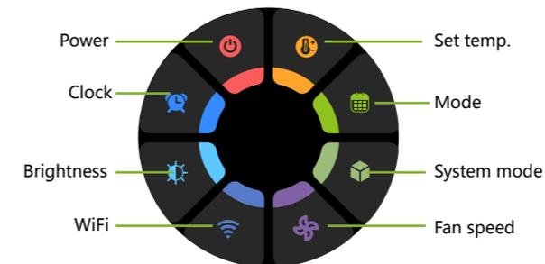
Tip: Press the screen to enter the Main control interface.
